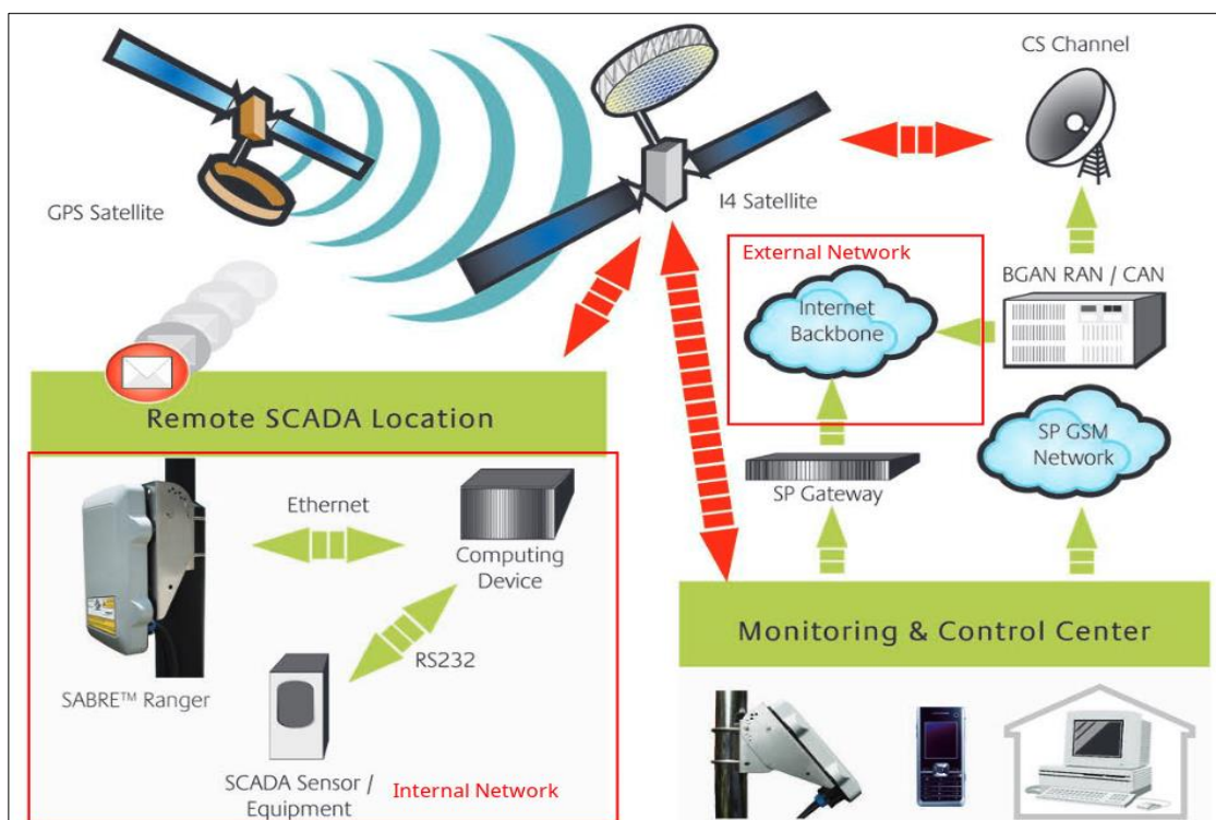
Figure 2. SATCOM Terminal Network Diagram
