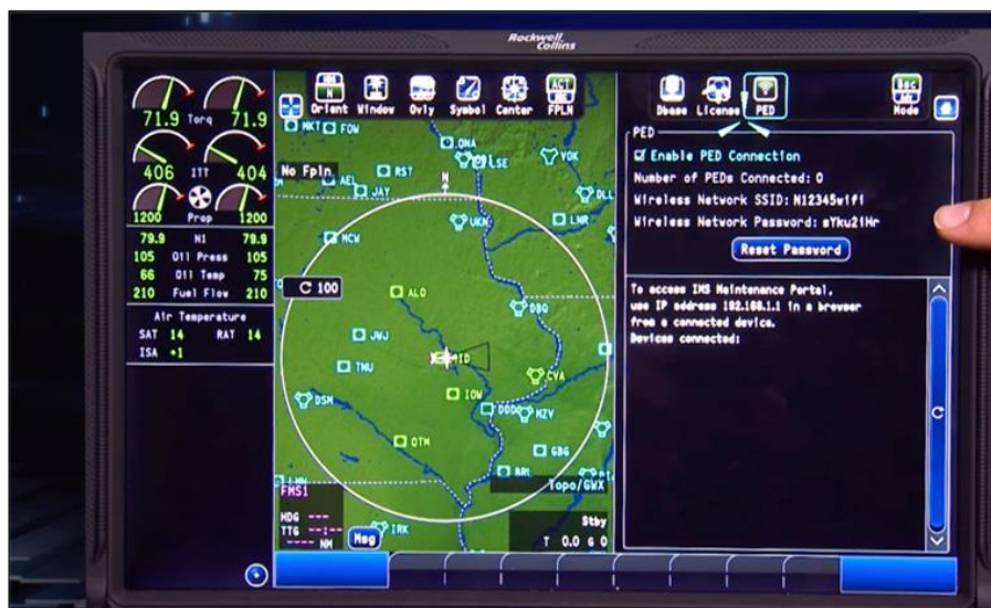
Figure 86. WiFi Enabled for IMS Maintenance Operations 46
